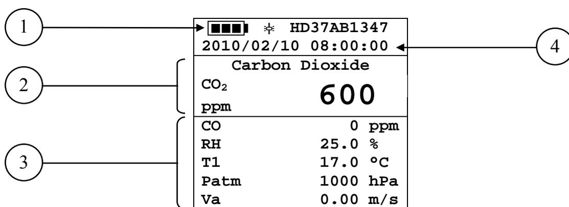
1. **Battery's charge status and instrument code.** In case the **logging** function is on, this line shows the current logging number and the time elapsed from logging start.
