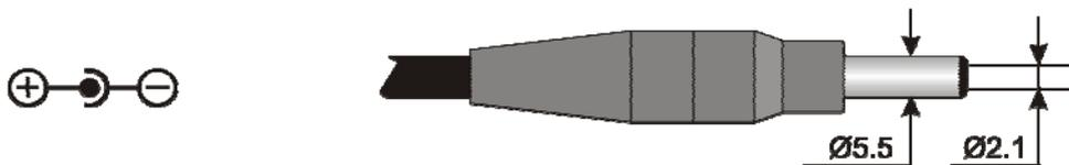
The external power supply connector has an external diameter of 5.5mm and an internal diameter of 2.1mm.
