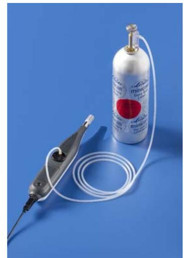
2. Let the inlet open if you want to perform a calibration at 400 ppm: For this second calibration procedure, **ensure the instrument is really in clean air.**
