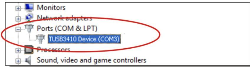
When the USB cable is disconnected, this item disappears and comes back when it is connected again.
